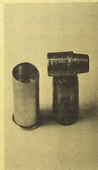
Core moved forward in recoil. Jacket stayed in place.
