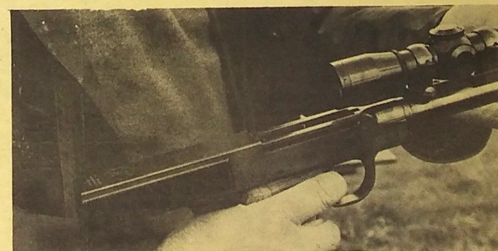
Action of the Kengill. It's a single shot. Simply drop the round in the top and close it to shoot.
