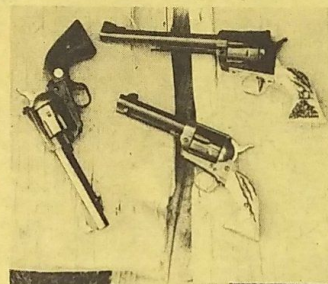
The most popular and probably most useful .45 Colt caliber revolvers are Colt and Ruger. The S & W's thin cylinder walls prohibit loading them to much over factory pressures safely.
