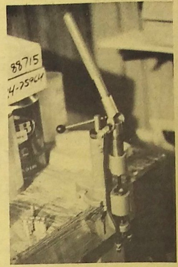
The RCBS unit is affordable, does a good job and will accept Lyman sizer dies and top punches.
