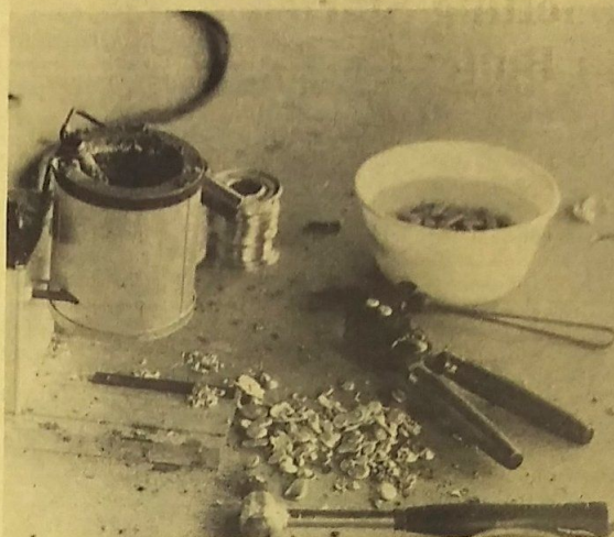
Dropping a hot cast bullet from the mould into water . . . doubles the hardness of the lead. Warning! water, or a wet bullet dropped back in the pot gives off a violent reaction spuing hot lead all over everything and everybody.
