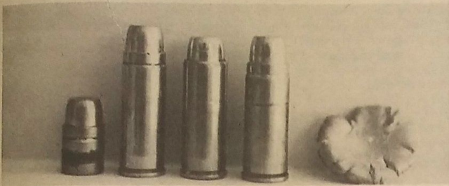
NEI 310451, loaded in .45 Colt trimmed by .050", over shoulder in .45 Colt case, in .45 Special case, expansion of Heavyweight .45.
