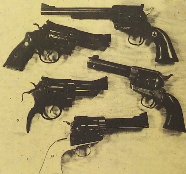
Some of the test guns. Top: 7.5" Ruger Flattop .44 Mag, 4" M29, 4.75" SA Colt, S & W 1950 Target and Custom Ruger.
