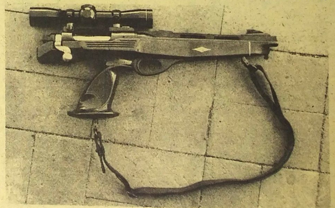
Web Sling and QD Swivels is one of the best ways to carry the big pistols afield.
