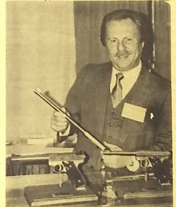
The AMT Ruger copy in bull, standard, and a long barrel assembly.
