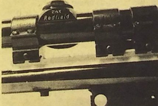
A close-up of SSK's Magnum-Proof scope mounting system.
