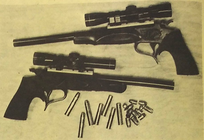
Top gun Super 14 .44 Magnum rechambered to .430 JDJ, SSK mounts, Leupold M8-4X. Bottom gun: Custom SSK .430 JDJ barrel, SSK mounts, Leupold M8-2X.
