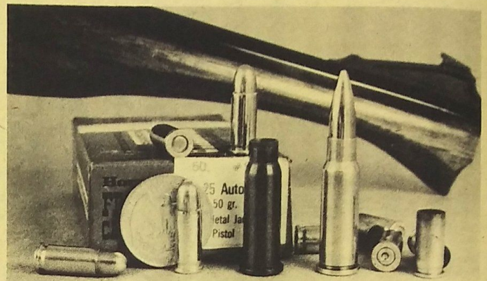
The anemic auto round, adapter and 256 Mag control load. T/C with Schiermier fore-end in the background.
