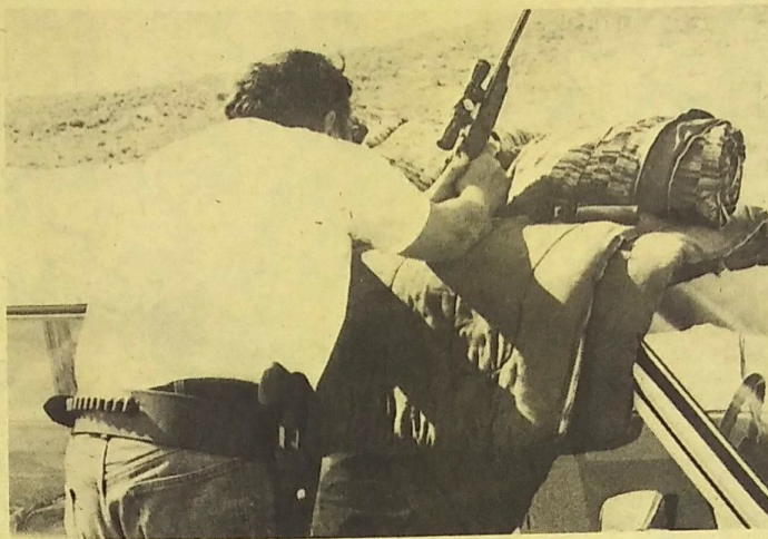
Full recoil of the 42-3031-350 grain load. Barrel is not yet ported. It definitely bounces, but isn't uncomfortable to shoot.
