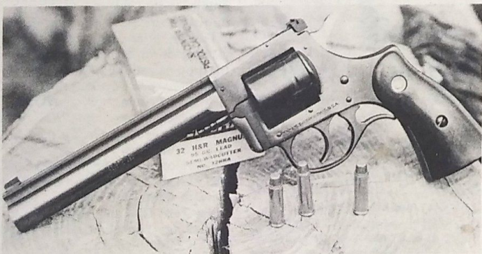
The H & R 504 32 Mag. is a lightweight, adjustable sighted five shooter. The ammo shown is 95 grain lead. Federal has a new 85 grain jacketed HP on the way.
