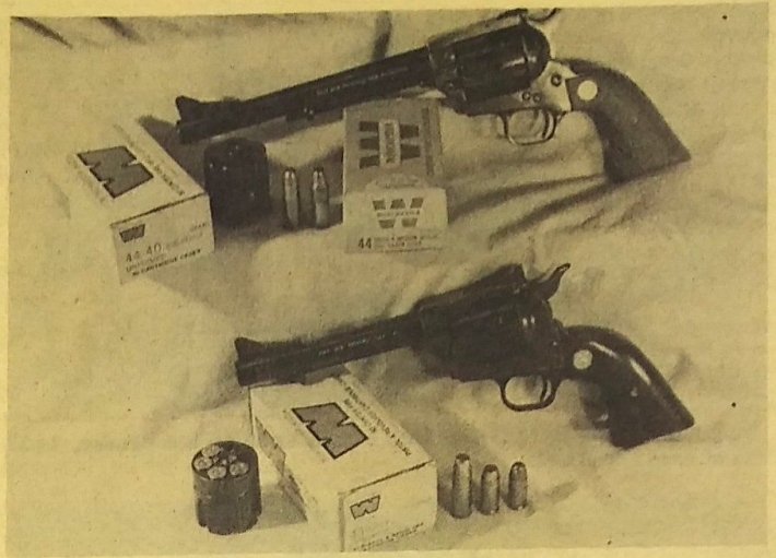
Colt New Frontier versatility. Top .44 Special and .44-40. Bottom .45 Colt, .45 ACP, .45 Auto Rim.
