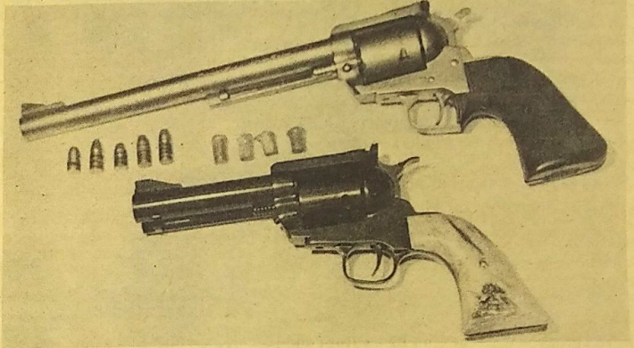
The 10" Custom Ruger and 4-5/8" Abilene. Both show extreme accuracy with heavy cast bullets. Bullets shown are a variety unfired and recovered. Action, very tight and perfectly timed.
