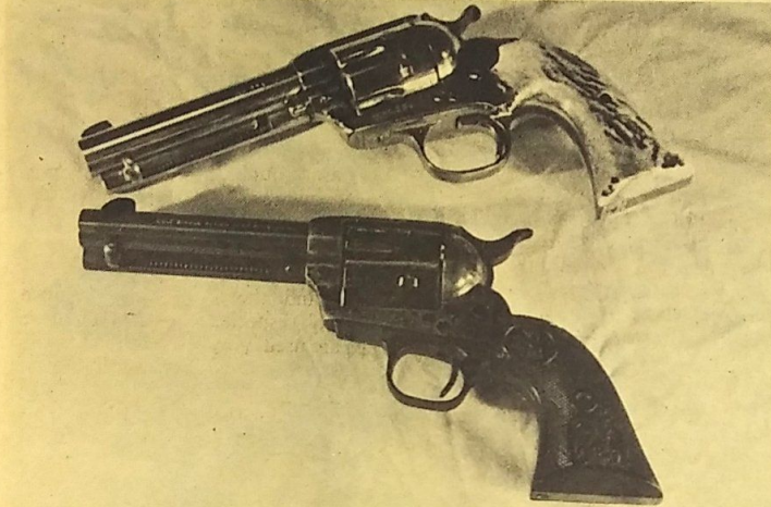
The grip shape of the Colt Bisley (top) and hammer are different from those used in the S.A. Army.
