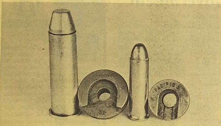
Everything about the .50-70 is outsized — even the shellholder. The little round on the right is a .357 Mag.
