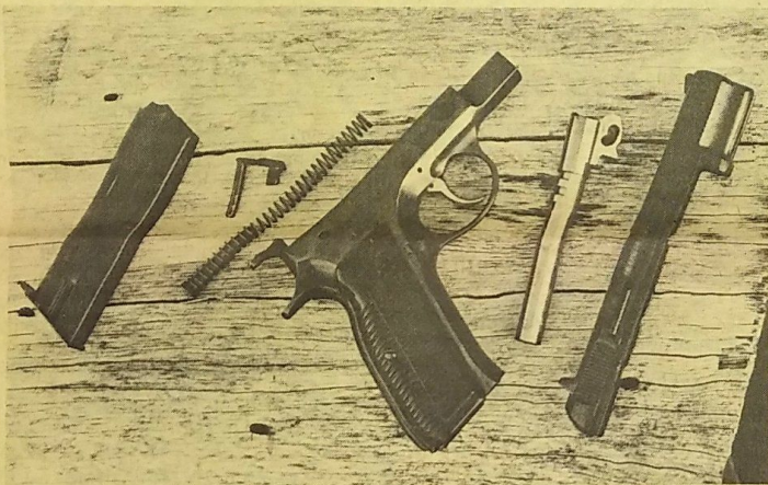
That's it! Not much to field stripping the CZ. Note differences in barrel from Colt and Browning.
